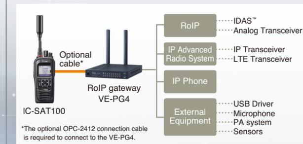
\*The optional OPC-2412 connection cable is required to connect to the VE-PG4.
